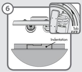
Installing the globe (sold separately) Position the indentations in the outer rim of
